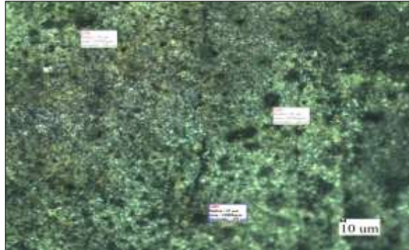
Fig. 9. Microstructure of brine tempered EN19 Steel Alloy (100x).
