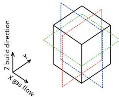
**Figure 2.** Cutting planes used for samples preparation.
