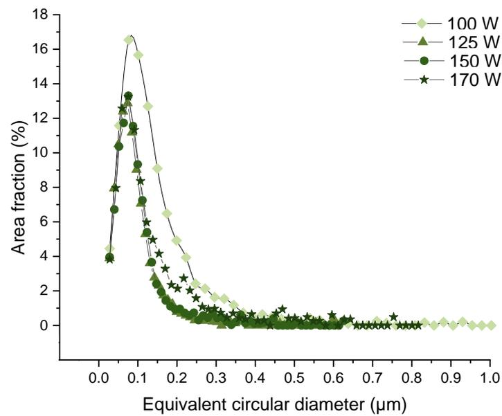
**Figure 10.** Power-dependent size distribution of spherical precipitates.
