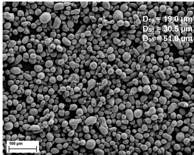
**Figure 1.** Powder morphology observed with SEM with powder size distribution reported.
