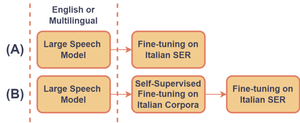
Fig. 3. Fine-tuning scenarios evaluated in this work: (A) The speech model is directly fine-tuned on the Italian SER task. (B) The speech model is first fine-tuned using an SSL approach on a large Italian audio corpus before being fine-tuned on the Italian SER task.
