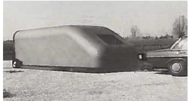
Figure 13. Trailer used to determine the rolling resistance of a vehicle [11]
