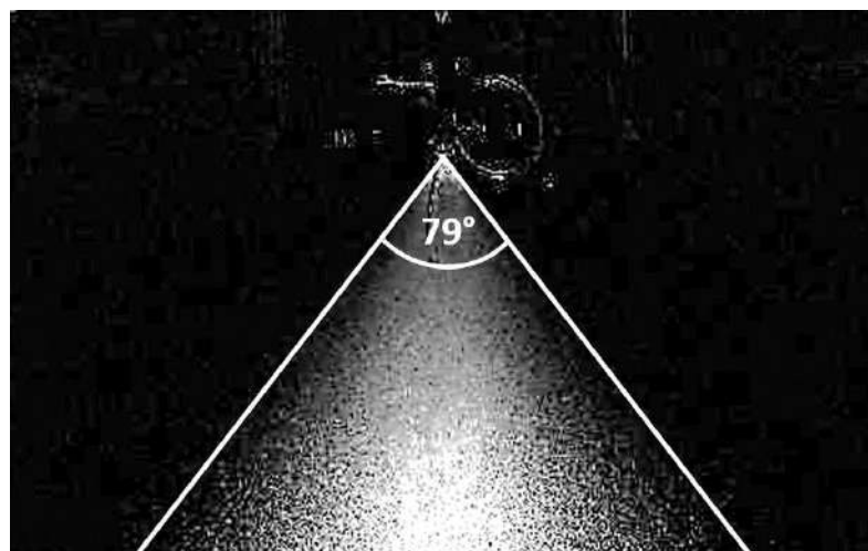
Figure 17. Hollowcone angle for a pressure of 2 bar measured during the experimental campaign.
