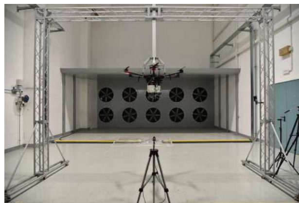
Figure 1. UASS and camera setup in the SEASTAR wind tunnel.
