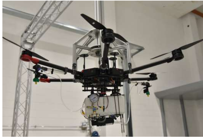
Figure 2. DJI Matrice 600 with customized spray system.
