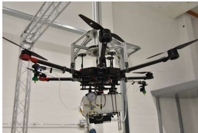
Figure 2. DJI Matrice 600 with customized spray system.
