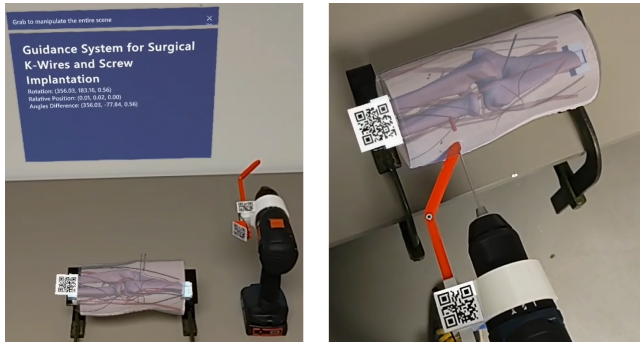
Figure 9: Guided K-wire Insertion in a Dummy: Virtual Overlay Revealing Internal Structures with the K-wire Tip Indicated by a Red Cylinder. Tracking achieved via QR code mounted on the drill, utilizing Vuforia™Instance.
