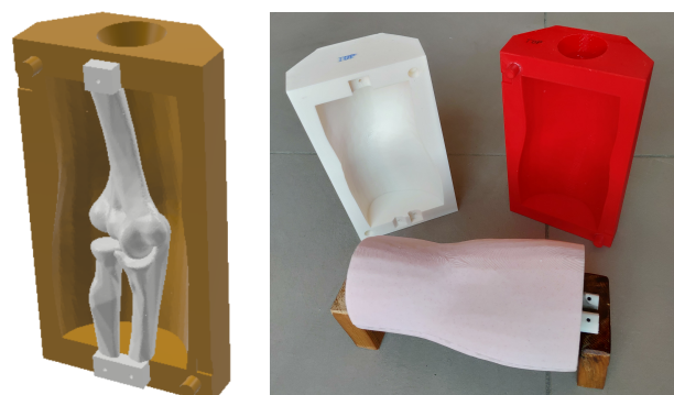
Figure 6: Left: rendering of humerus, radius and ulna with negative soft tissues mold (side B); Right: physical phantom on wooden supports and molds (from left to right: side A and B)
