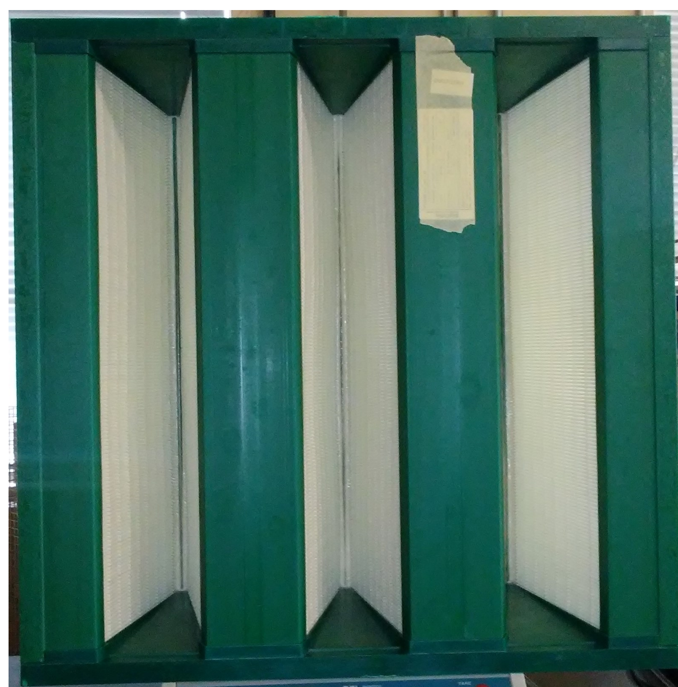
Figure 4. Compact filter tested made up of fiber glass.
