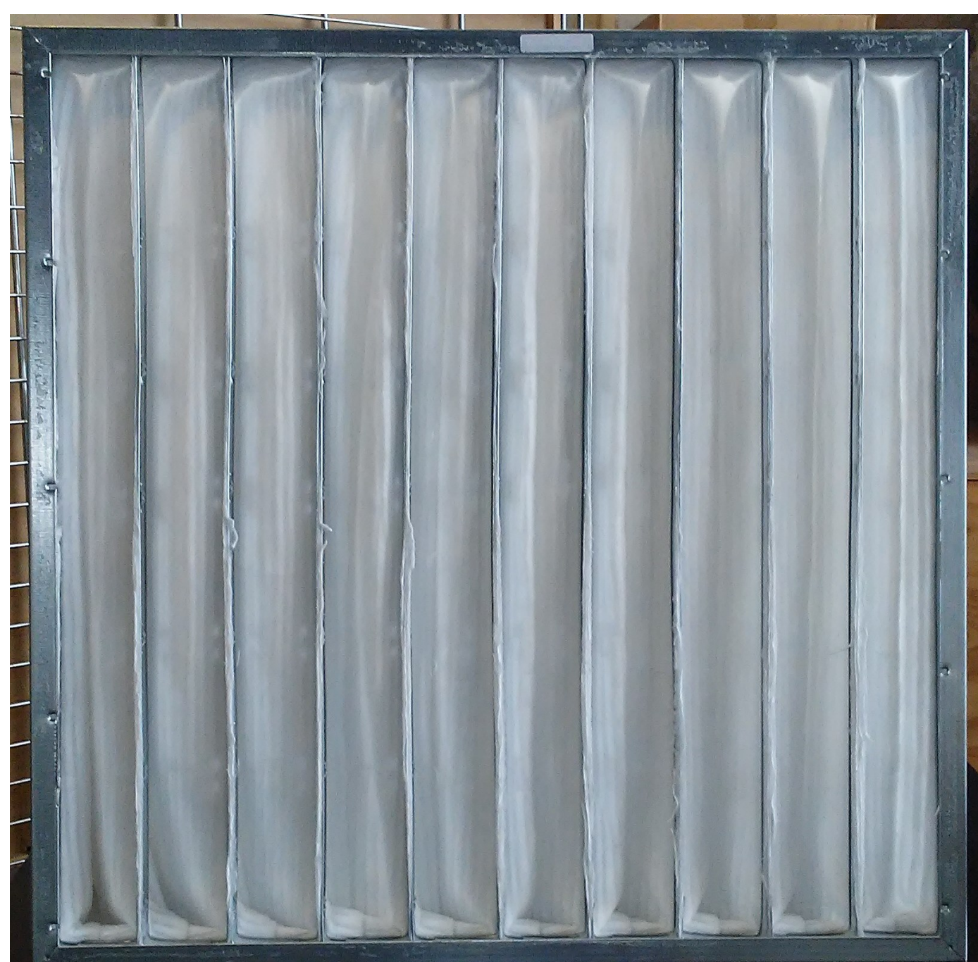
Figure 3. Pocket filter tested made up of synthetic material.
