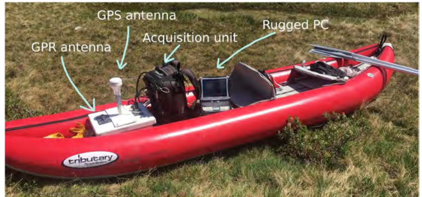
FIGURE B2 The inflatable boat carrying the GPR system. All components are ruggedized and protected from water splashes
