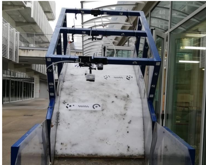
Figure 31. Snow melt experiment on the Laboratory Landslide simulator. GoPro cameras attached on the frames above the snow.
