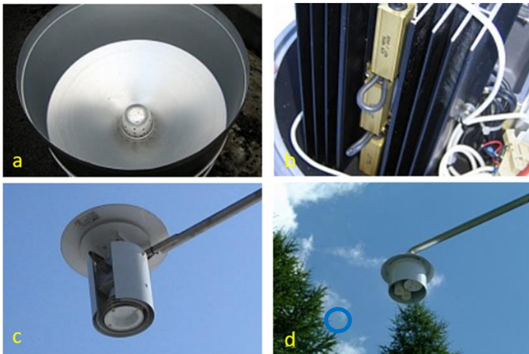
Figure 19. a: Bascule Rain Gauge conveying mouth; b: Bascule Rain Gauge heating system; c: Thermo-igrometer measuring Temperature and Relative Humidity; d: Ultrasonic sensor for Snow depth recording.
