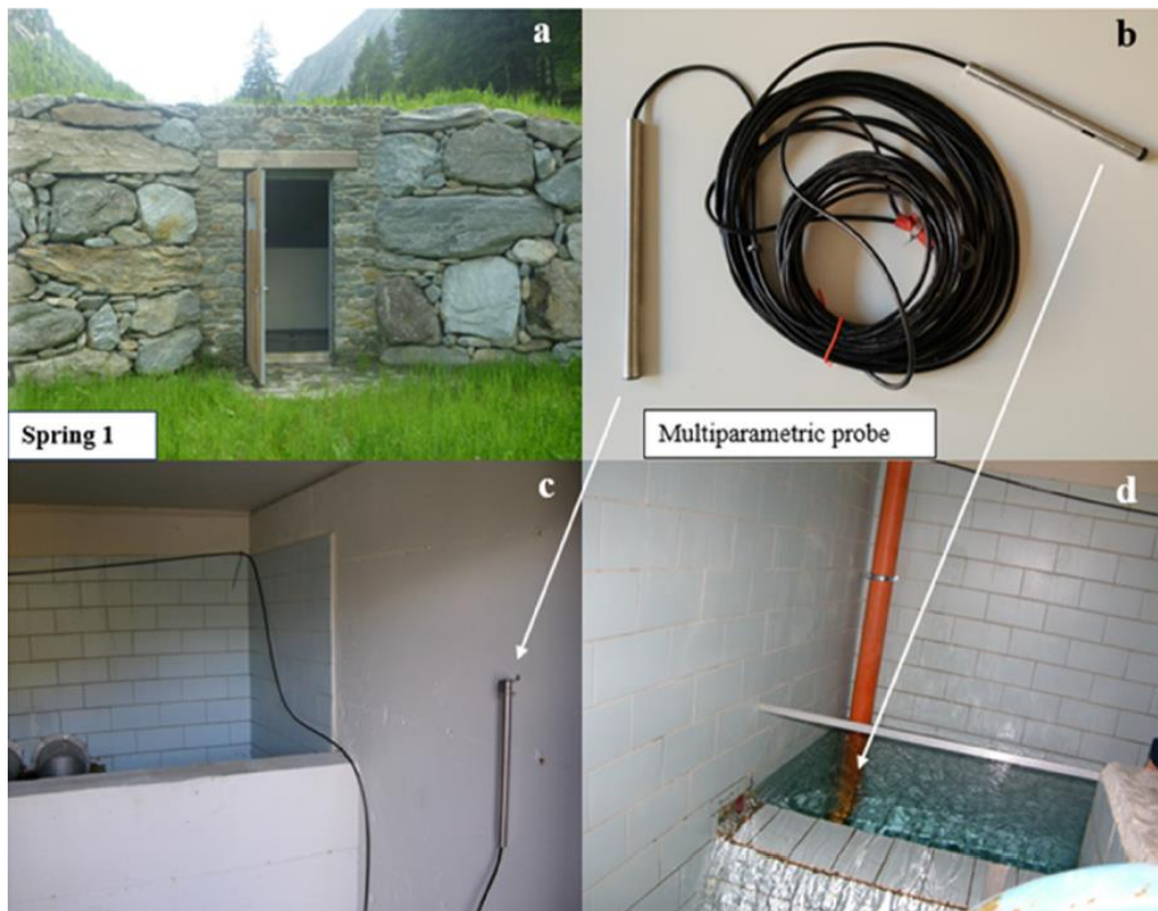
Figure 22. Typical set-up of a monitored spring (Mondani, Gizzi and Taddia, 2022).
