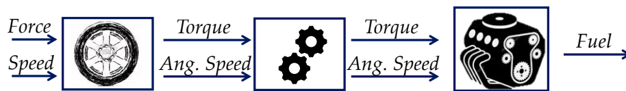
Fig. 4.2 Information flow in a backward kinematic approach.
