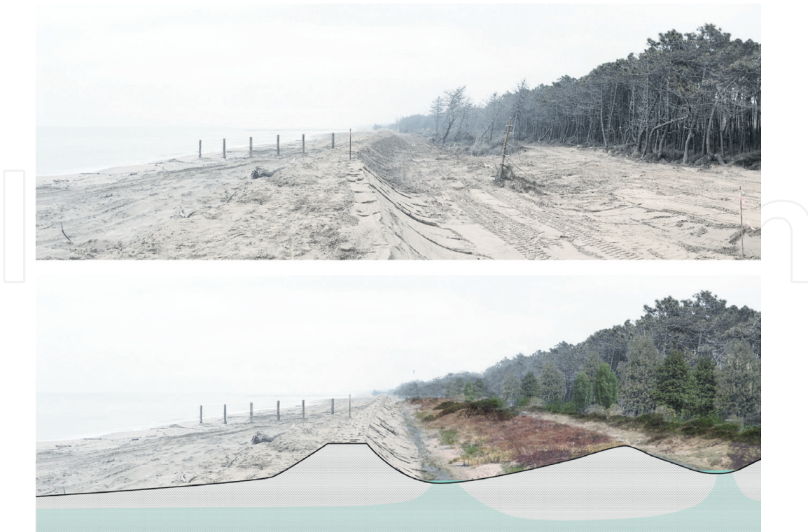
Figure 5. Critical coastal area (actual situation); design arrangement for dynamic shoreline stabilization. Source: author, from SECAP 2020 Ravenna Authors. SECAP Ravenna 2020.
