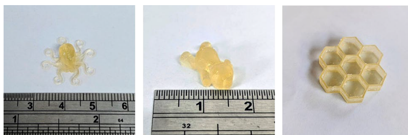
Figure 11. 3D-printed specimens produced from the 3SH-IsDPC formulation under the optimized DLP printing conditions.
