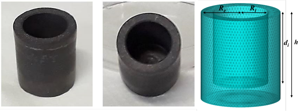
Fig. 3.3 Picture of the cup-shaped MgB 2 shield (left and center) and its schematic view (right). Its dimensions are: inner radius R_i=7.0 mm, external radius R_e=10.15 mm, external height h_e=22.5 mm, internal depth d_i=18.3 mm.
