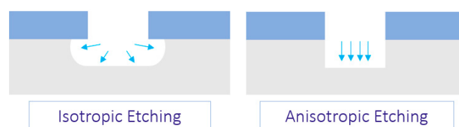
Figure 7. The isotropic and anisotropic behavior of wet- and dry-etching.
