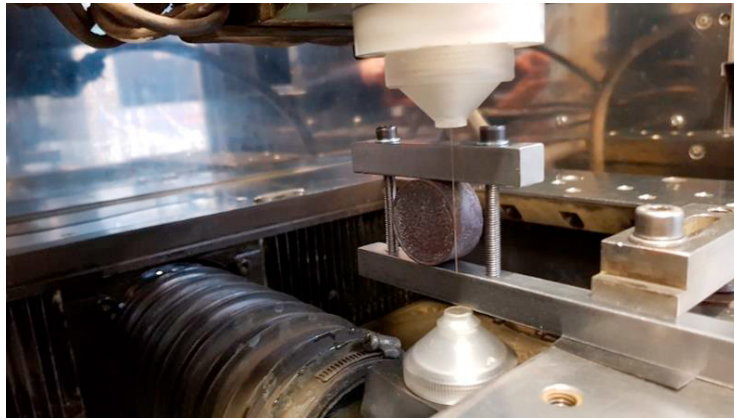
Fig. 1 Production of discs by cutting with EDM technique.
