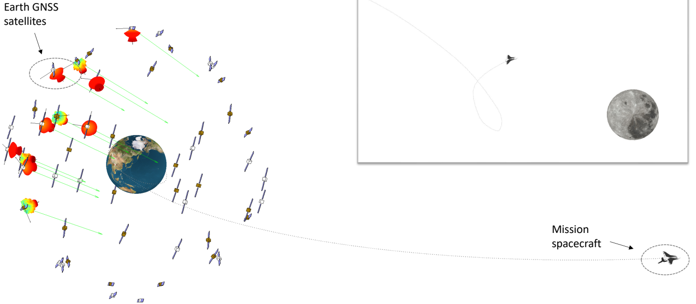
Fig. 2: Snapshot of the mission-case scenario as reproduced by the custom Matlab ® -based mission planner and GNSS constellation simulator. Transmit-antenna radiation patterns are shown for satellites in radiometric visibility from the spacecraft. Vectors pointing towards the spacecraft are shown as well.
