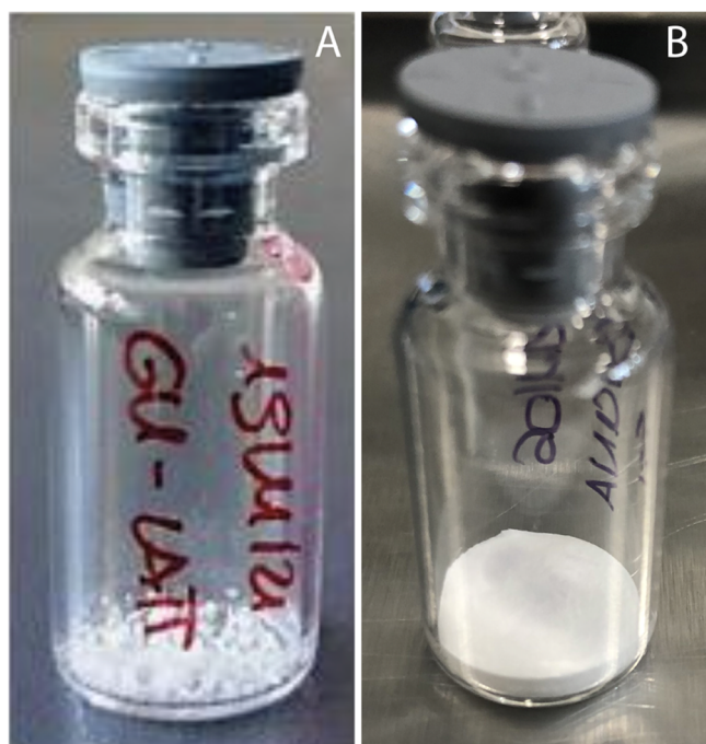
Figure 3. Representative images of (A) collapsed (EVs with lactose and glycine) and (B) good (EVs with glycine 5%) structure of the lyophilized cakes.
