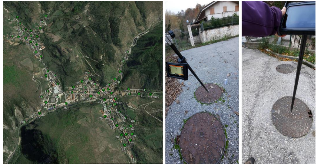
Figure 7. Some examples of Ground Control Points (GCPs). On the left the reference points are numbered in green in the KML file, on the right two photos of the GNSS instrument during the survey. Source: Flyengineering s.r.l.
