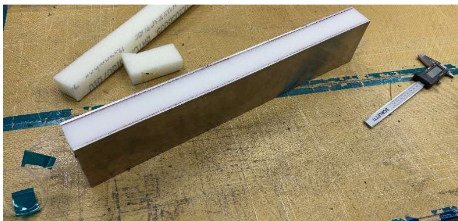
Figure 51: manufactured beam specimen (B02) after mechanical pressing.
