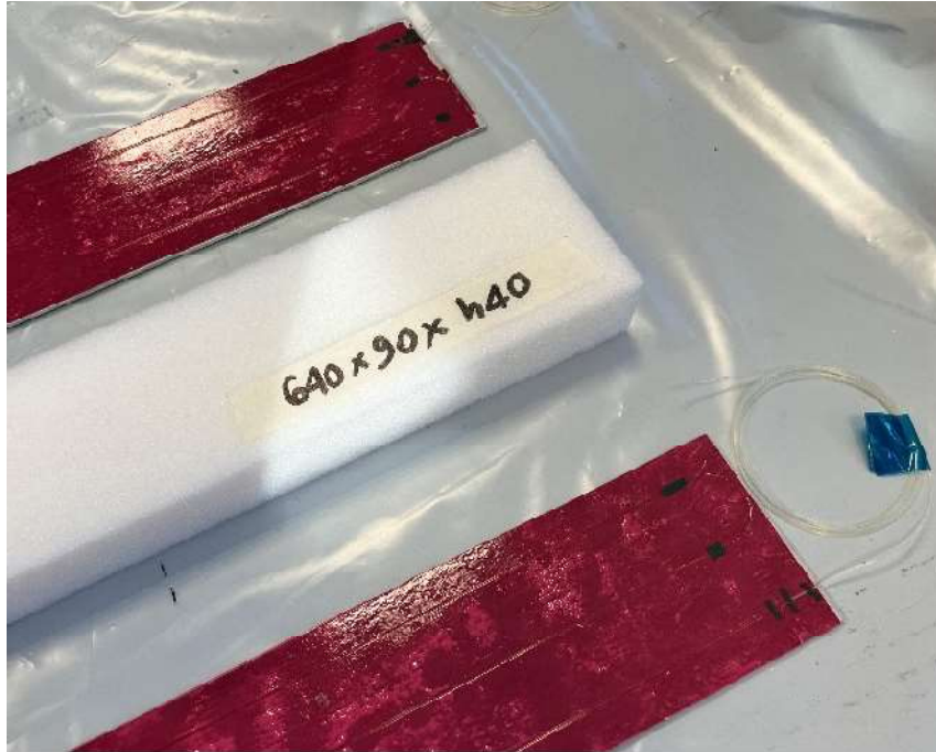
Figure 50: fibre optic sensors placed on the Ergal face-sheets, adhesive layer (in red) and Rohacell® IG-31 foam.
