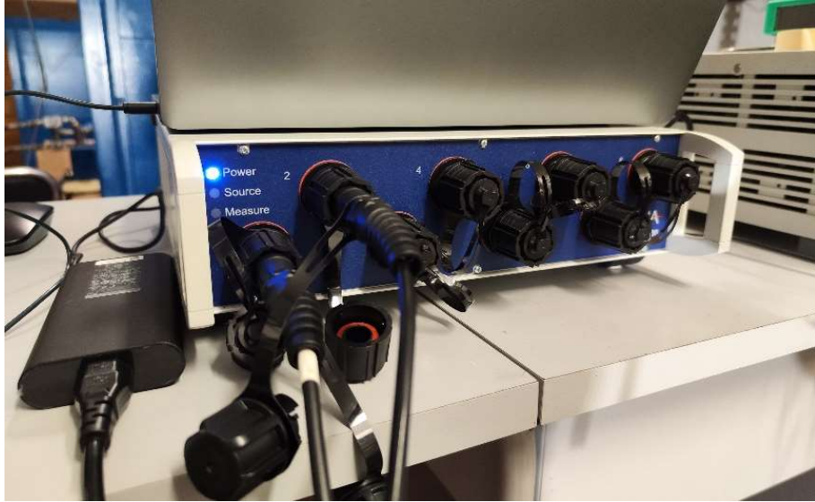
Figure 52: Luna Inc. ODISI 610x optical fibre acquisition system.
