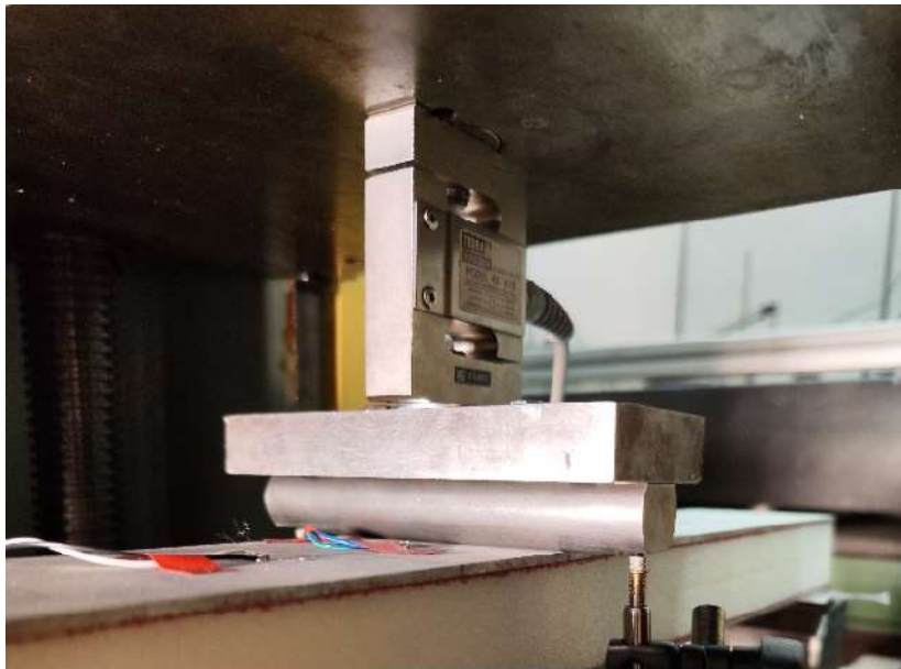
Figure 53: HBM strain gauge load cell (200kg)
