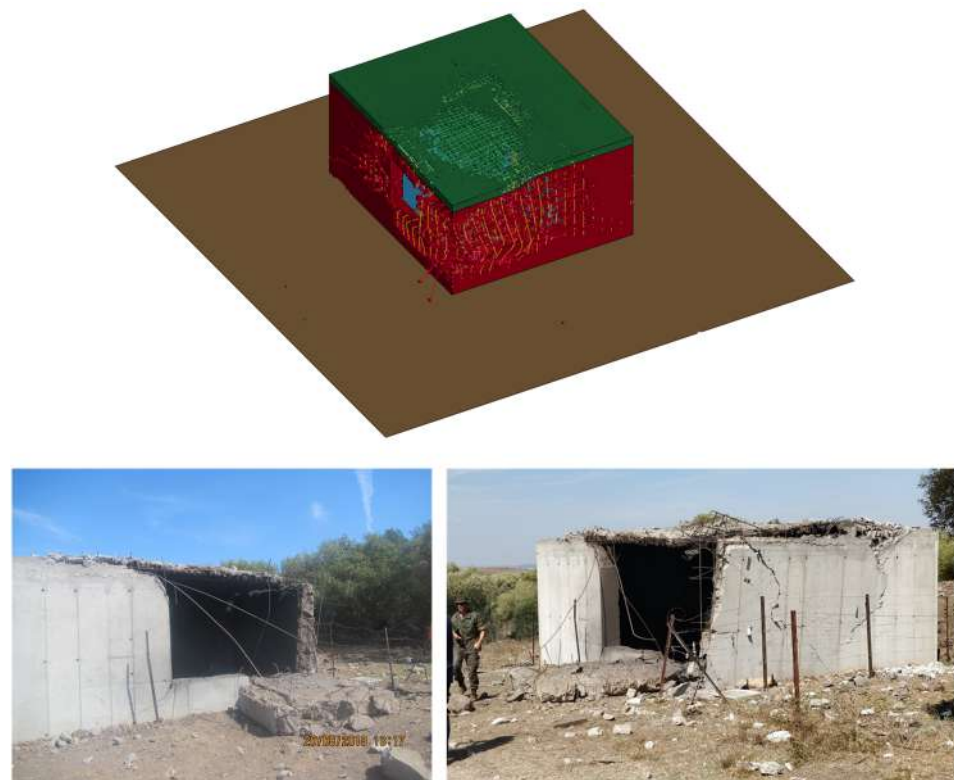
Figure 12. Final test (T8) results: numerical model and photographs.
