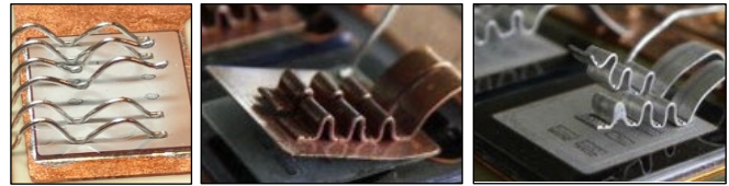
Fig. 1. Thermo-mechanical failures of state-of-the-art power semiconductor interconnects [3].
