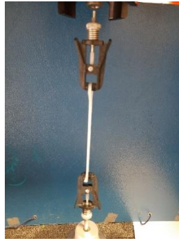
Fig. 1.20: The mechanical tensile strength test.
