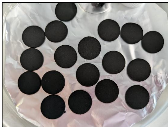
Fig. 2.3: Self-standing porous AC electrodes
