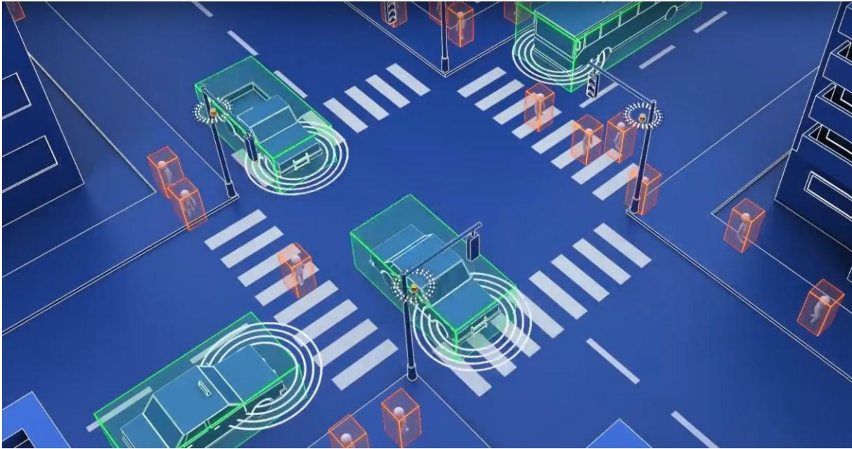
Figure 6. Road users' recognition and classification into cars, heavy vehicles, bicycles, and pedestrians.
