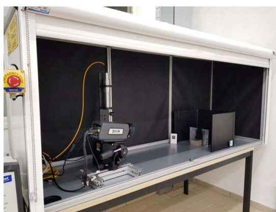
Fig. 3 – Active thermography test bench.
