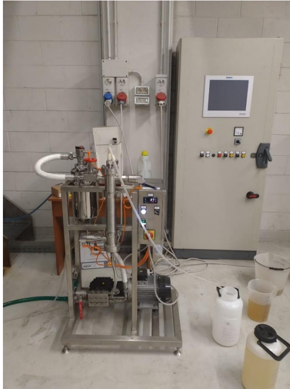
Figure 3.6: Pilot membrane filtration plant
