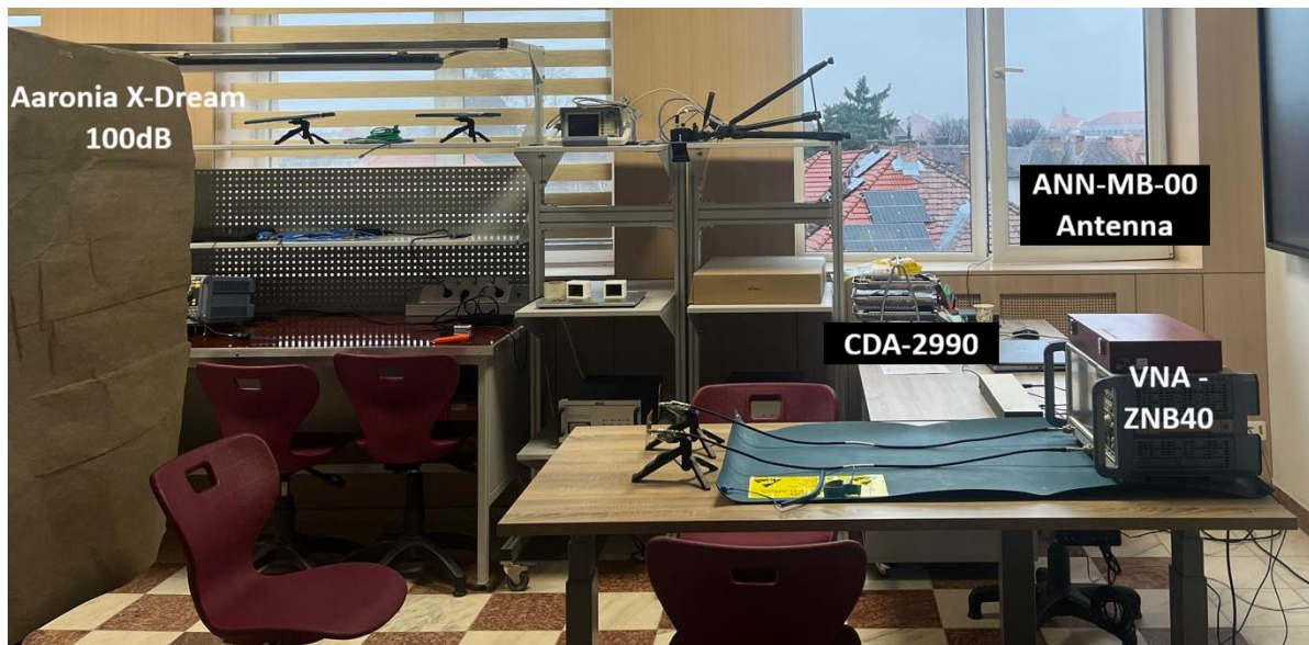
Figure 13. Experimental setup used for the comparative analysis of antenna sensitivity in vital signs detection.
