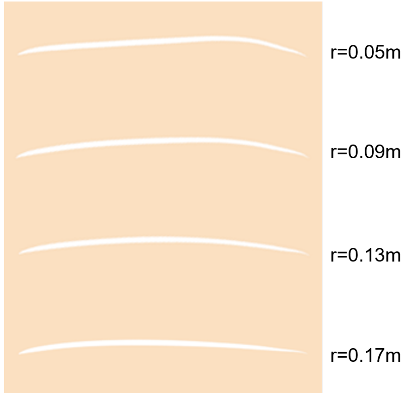
Fig. 10 Normalized airfoil sections at different radial stations after adjoint optimization. Two-bladed rotor.
