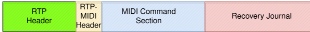
Fig. 4: High level packet structure, according to RFC4695. The RTP Header is the one described in RFC3550, without header extensions.
