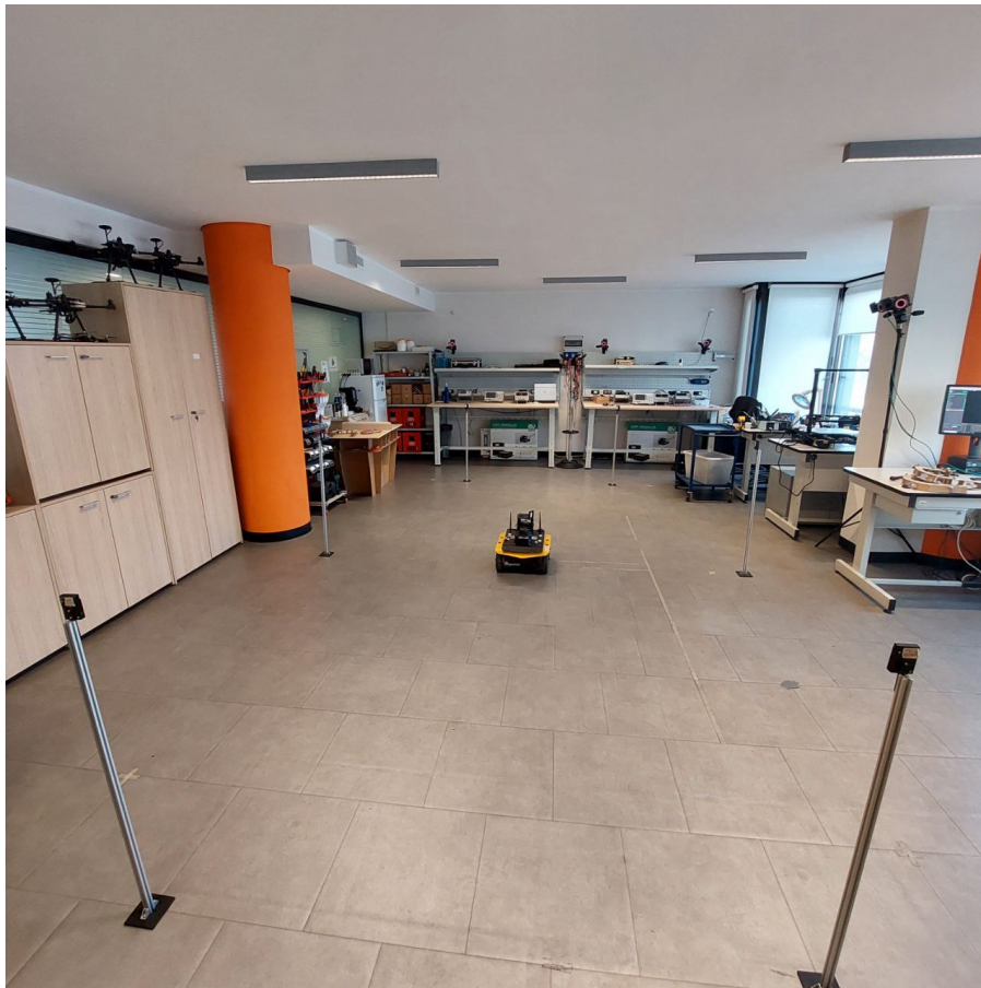
Fig. 4.11 The laboratory equipped with a Vicon tracking system and the Jackal rover used for the experiments. Obstacles are placed in different positions around the area to create the testing scenarios.
