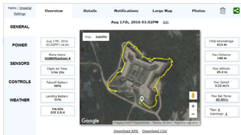
Figure 4. Example of flight path pattern for Prince of Wales Fort—Screenshot from airdata.com [23].
