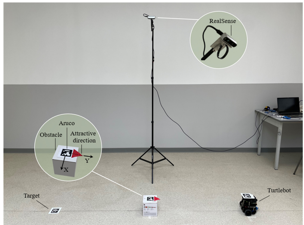
Figure 5. Laboratory setup. The Turtlebot, the obstacle, the target position, and the Realsense camera are highlighted.
