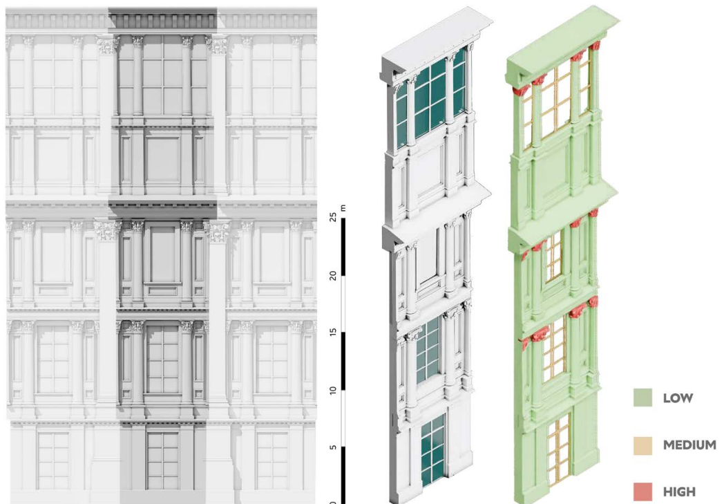
Fig. 5. Level of References - LoRef (from: Giovannini 2017) applied to the "dynamic model" elements. Elaboration by L. Torresi.
