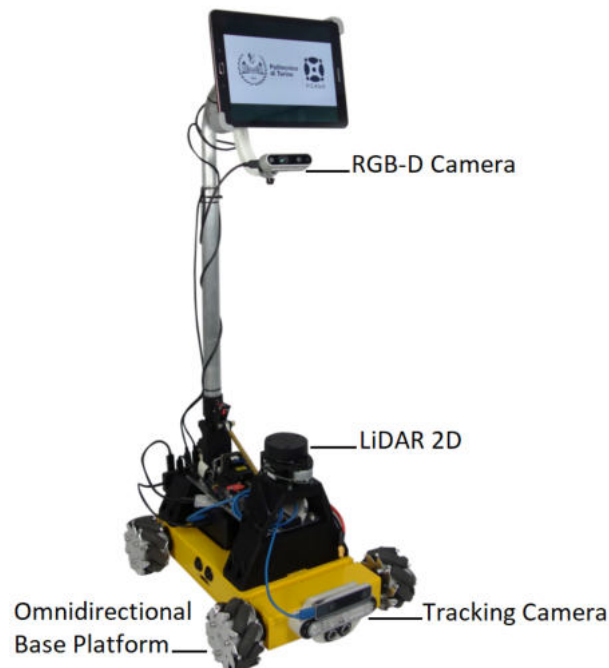
Figure 3. The omnidirectional platform we set up for experimentation and validation of our novel methodology. The vertical shaft allows the camera to be elevated over most indoor environment obstacles.
