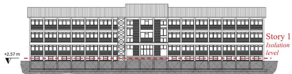
Figure 8. Position of the isolation level (red dashed line) with location of the single-concave FP devices.
