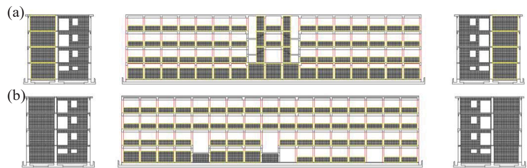
Figure 7. Identification of external totally and partially masonry infilled frames. Frontal and lateral views of the building (a); back and lateral views of the building (b).
