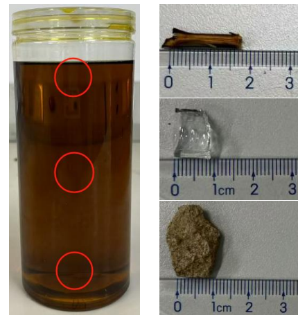
Fig. 12. The oil jar with contaminants considered in the experiment. The fragment of wood is placed on the upper part of the jar, the small splinter of glass is placed in the center and the stone is placed at the lower part.
