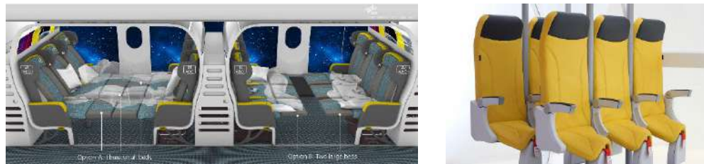
Figure 4. Reconfigurable (left DLR SL) and high-density seat configurations (right [9])
