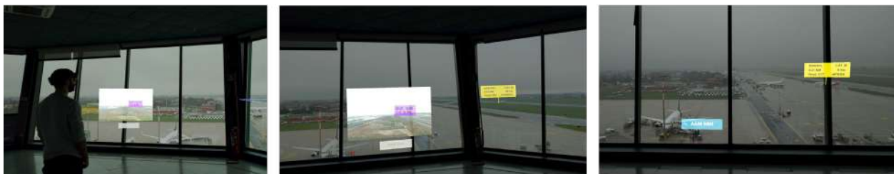
Figure 4 XR-based HMI for drone monitoring (virtual) integrated with a real-time AR interface for tracking airport traffic in Bologna airport control tower as visualized by a user wearing a Microsoft HoloLens2 devices.
