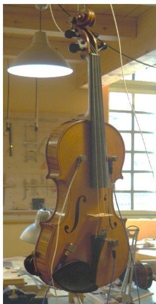
Figure 1. Set-up for the Modal Experimental Analysis.
