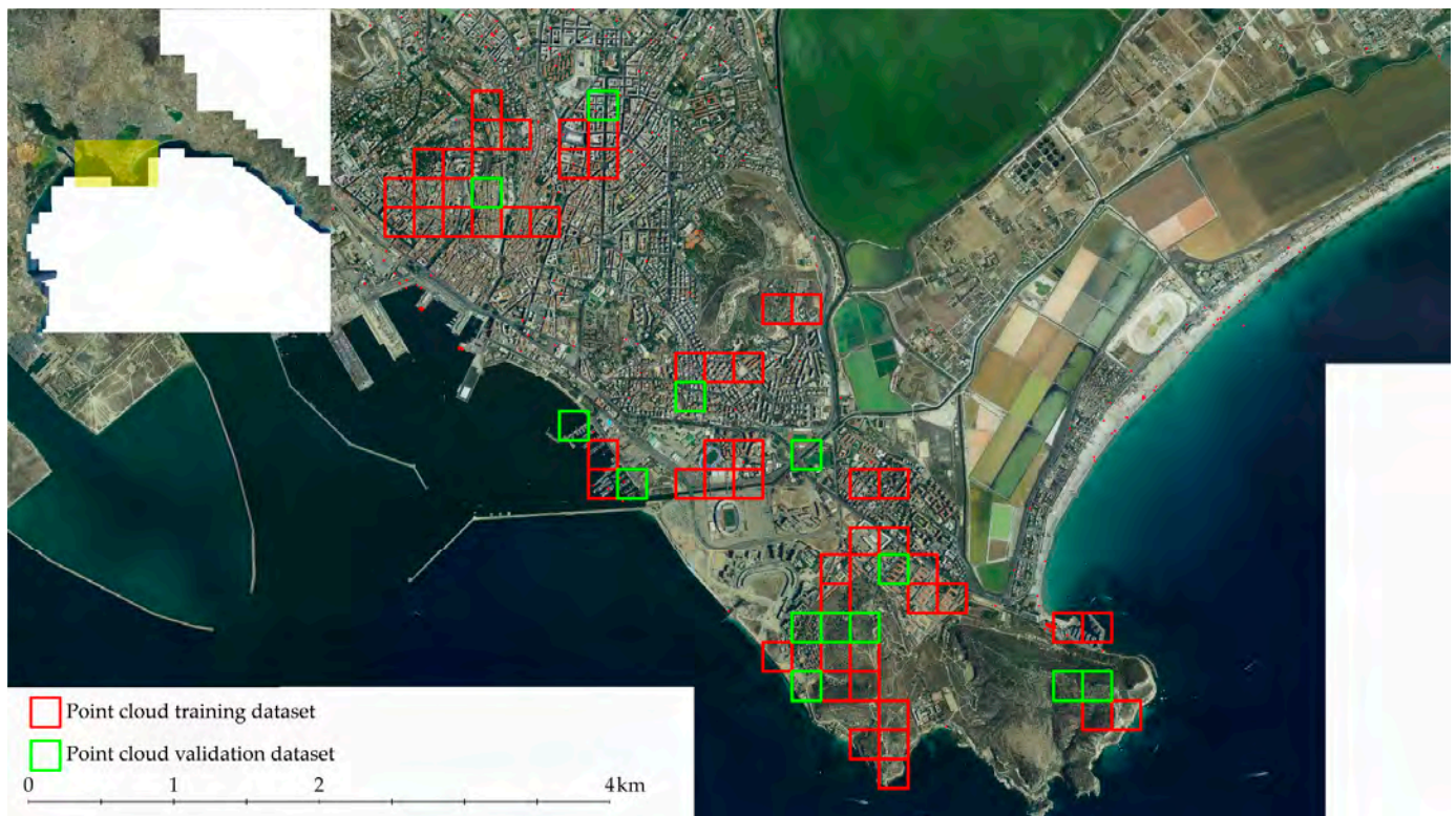
Figure 8. Map of the location of the training dataset (case study 1, Cagliari). The red tiles are about the training set, while the green blocks relate to the point cloud tiles used to validate the model.
