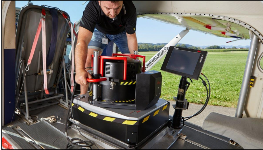
Figure 14: Leica Hybrid sensor on board aircraft used for the data acquisition for Torino DT project (Luigi La Riccia et al., 2024)
