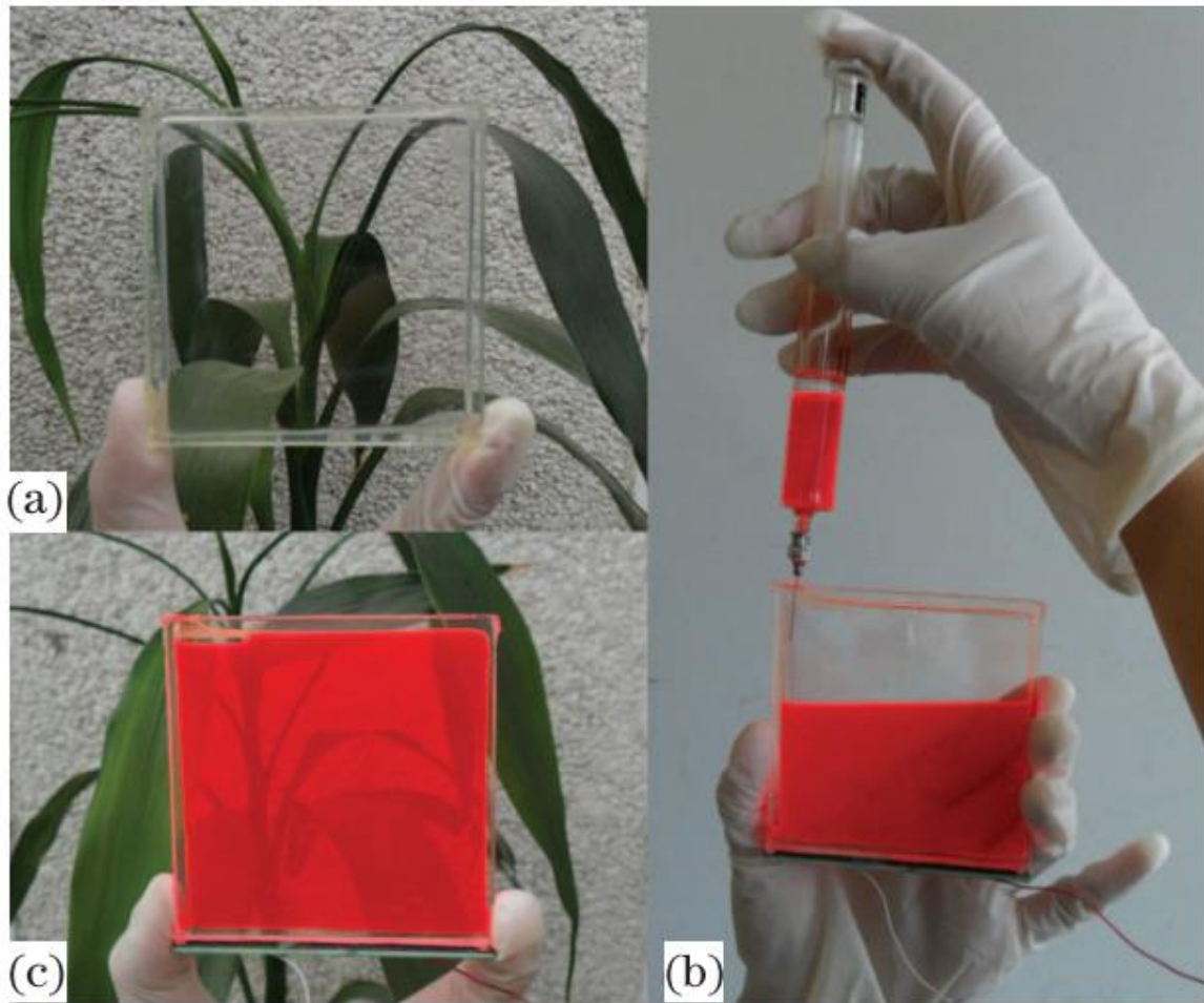
Fig. 3. Photographs of (a) the blank device, (b) the syringing process of fluorescent solution, (c) and the as-prepared aqueous layer LSC before the remaining three solar cells were attached.
