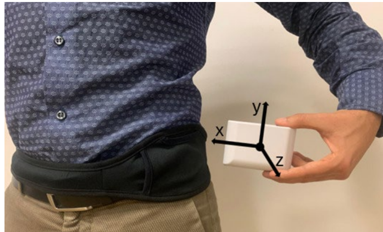
Figure 1. Wearable sensor (STAT-ON™) position and axes orientation.
