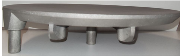
Fig. 4.37 3D printed prototype mirror after manufacturing and depowdering.
