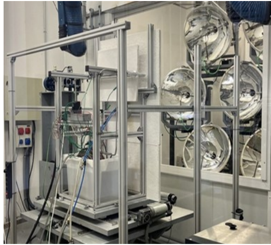
Fig. 3.3 The test table with the Xenon lamps. Taken from [106]
