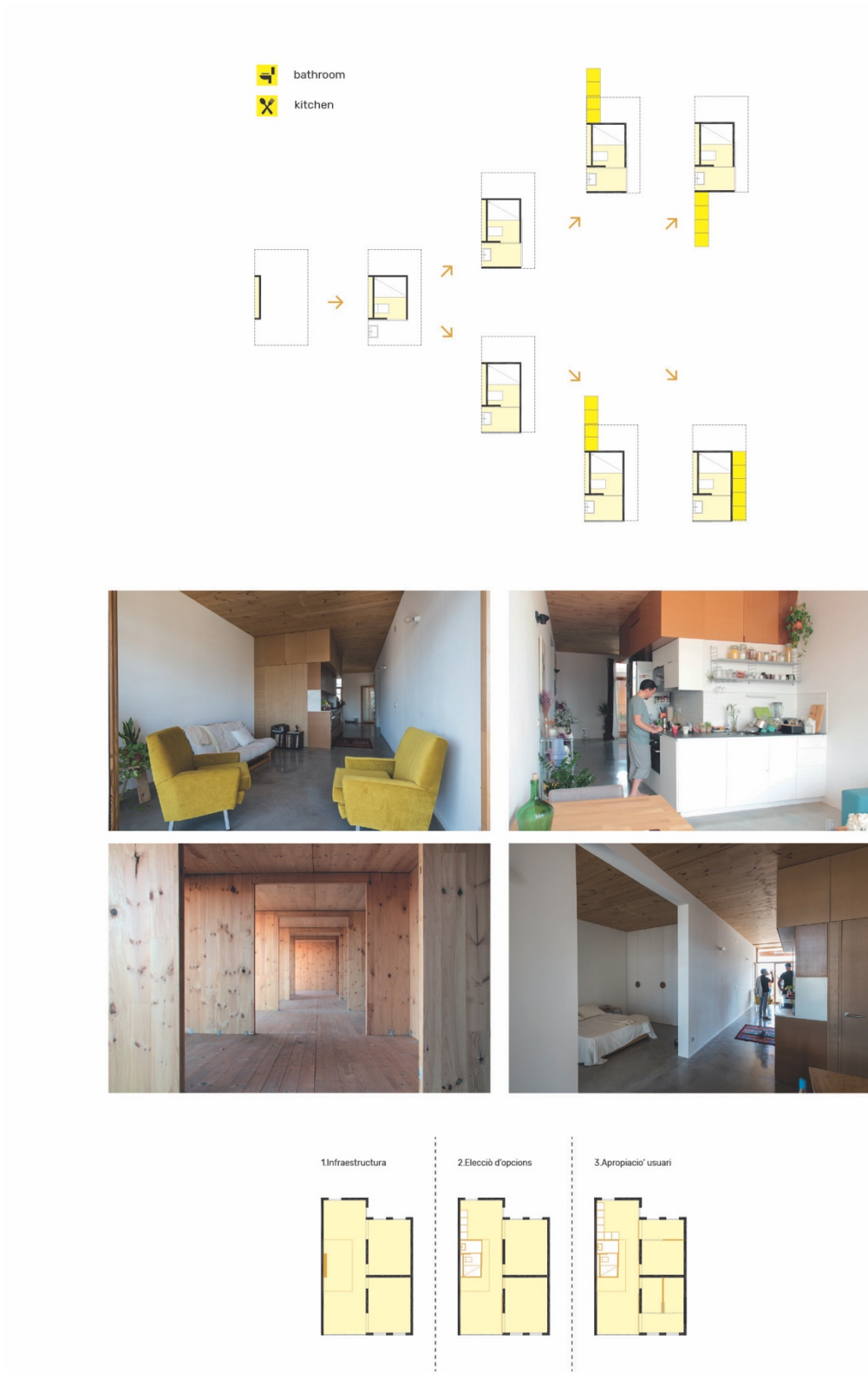
Fig 68: The flexible structure use; different compositions of the services spaces bathroom and kitchen. Drawing by the author; a study and elaboration from Lacol original drawings. Photos By Lacol Archive.
