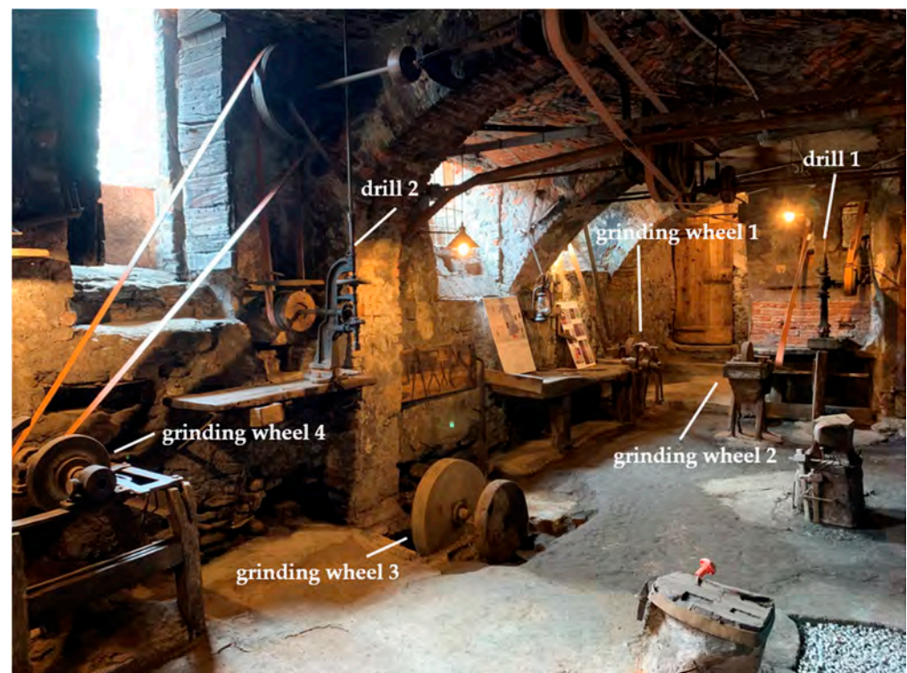
Figure 14. The machine tool apparatuses: two drills and four grinding wheels.
