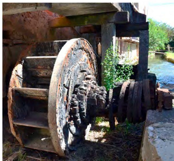
Figure 17. Water wheel #2 powering tilt hammer #2.
