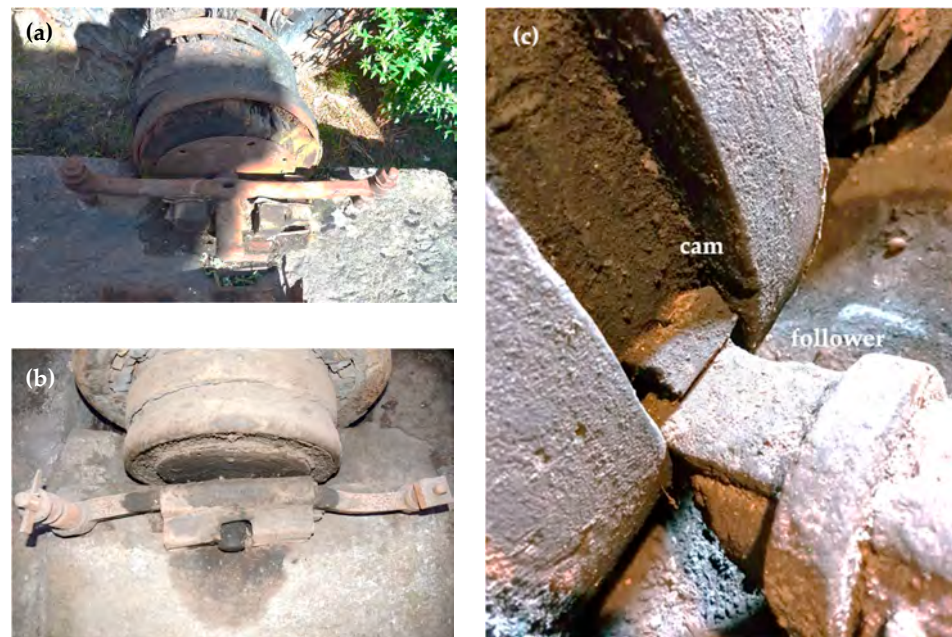
Figure 20. (a) External wooden plain bearing #1; (b) internal wooden plain bearing; (c) cam and follower.
