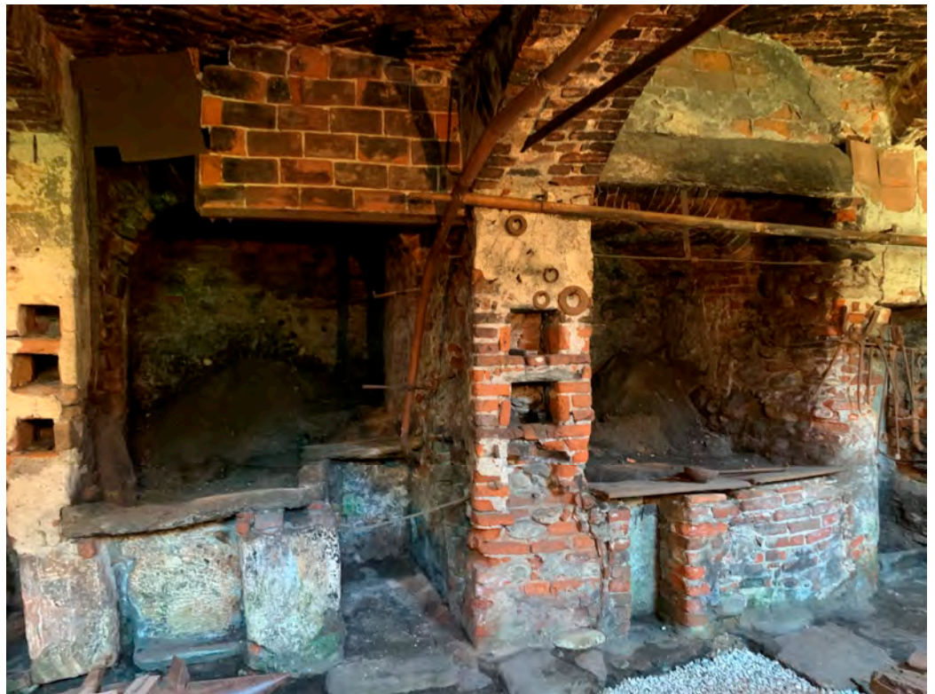
Figure 12. The forge. It is possible to see the old air pipes connected to the hydraulic trompe.
