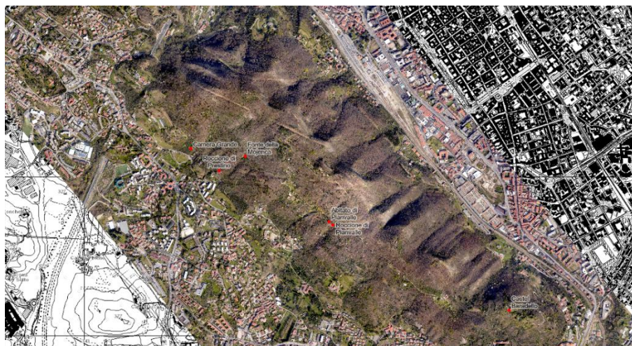
Figure 1. Map view from the GIS database of the park area, showing the high scale and high resolution orthophoto derived from ALS data based on the helicopter flight. Archaeological sites object of terrestrial image and range based 3D survey are highlight.
