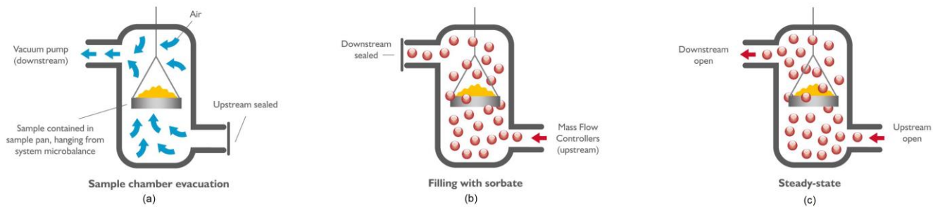
Figure 2. The dynamic adsorption measurement: (a) sample chamber evacuation, (b) filling with sorbate, (c) steady state (amount of sorbate molecules entering and leaving the chamber is controlled simultaneously) (after [46]).
