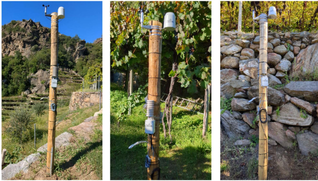
Fig. 1. Examples of weather stations used to acquire the dataset; the leaf wetness sensor can be recognized in the lower part of the pole.
