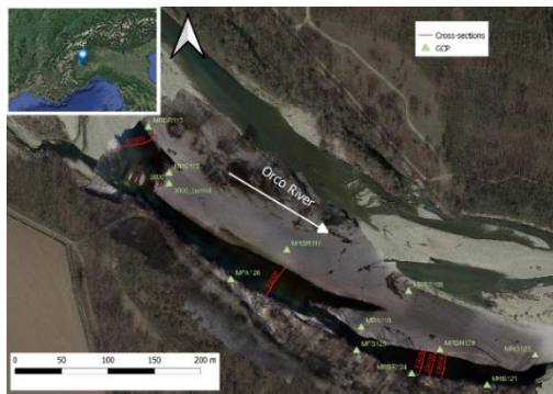
Figure 5. Orco river orthomosaic map. The red lines indicate the cross-sections measured with GNSS, while the green triangles are the GCP used in the photogrammetric procedure.
