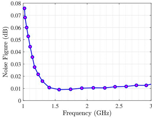
Fig. 4. NF specification of the LNA in [12].
