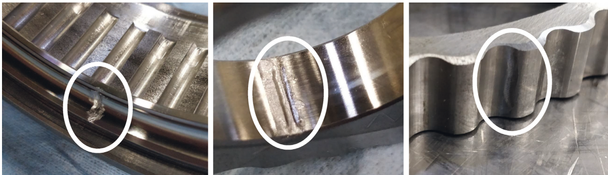
FIGURE 3: Gearbox artificial damages.
