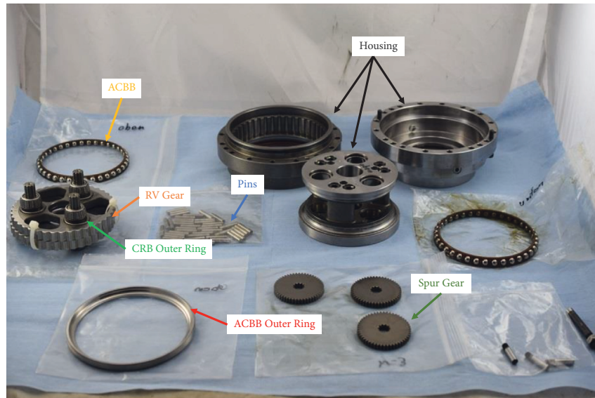
FIGURE 2: Dismantled nabtesco RV-42N.
